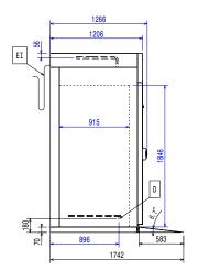
Electrical inlet (power) ΕI Refrigerant Outlet RO
